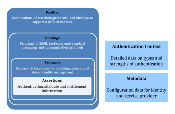
Figure 4.3. Basic SAML architecture (adapted from [40]).
